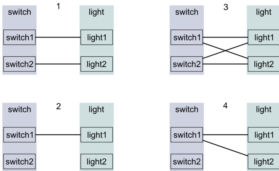
In the Weaver used, the combination policy between join points is number 3 of the figure above. All possible combinations are performed and the advice is duplicated as many times as there are combinations. In each instance of advices, the weaver replaces variables representing the components by the value of the combination.
