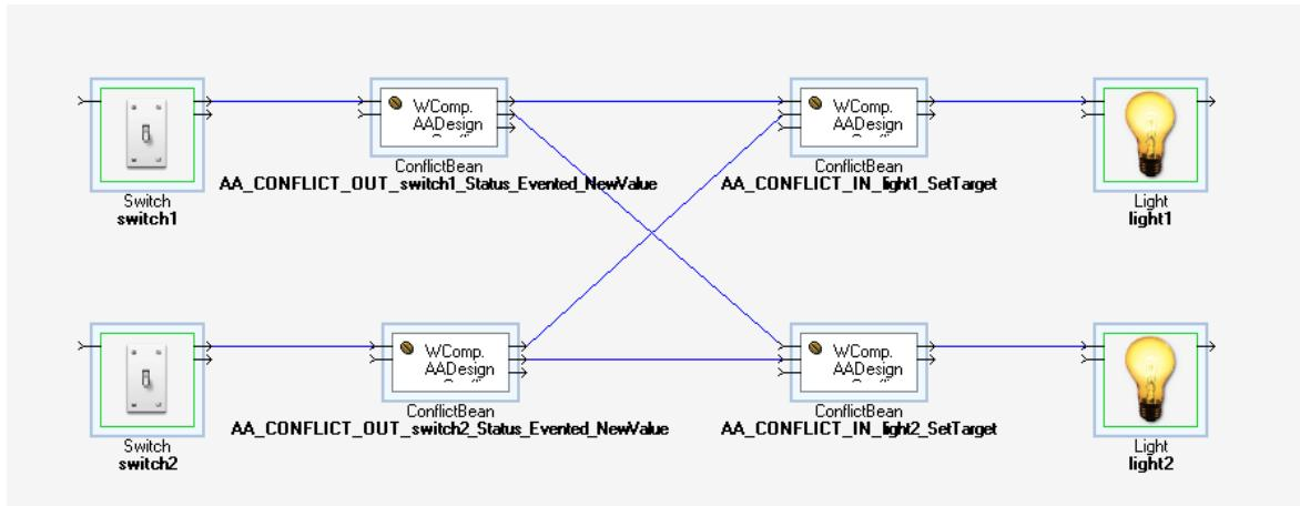
These components symbolize the detection of a possible conflict between two links of the assembly, after adaptation of the application. They currently have no effect on the progress of the application, but will eventually replace to merge advices in a specific way.
