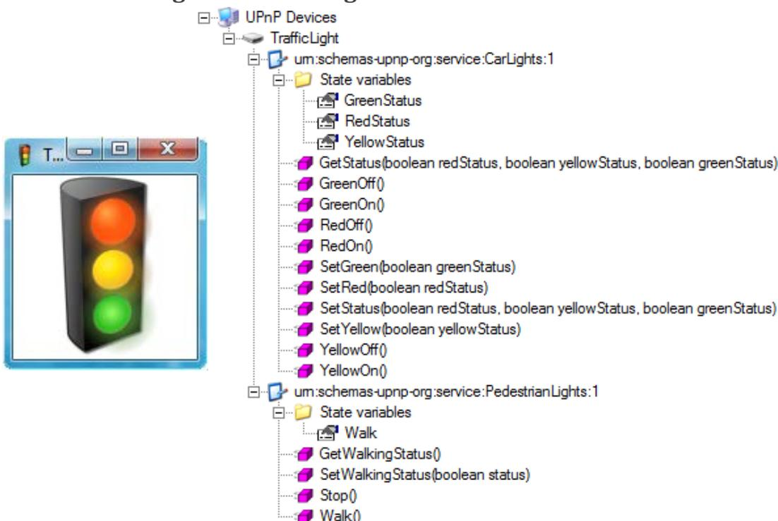
Figure 1: UPnP Interface of the Traffic Light Device
