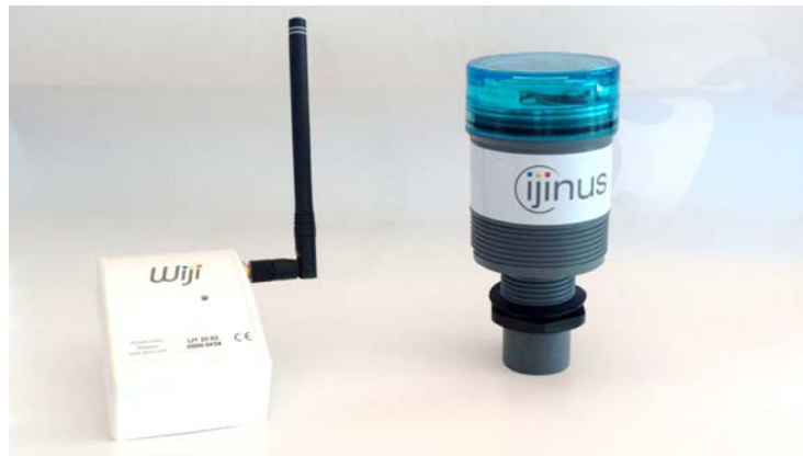
Figure 3: Ijinus ultra sonic sensor used as validation prototype.
