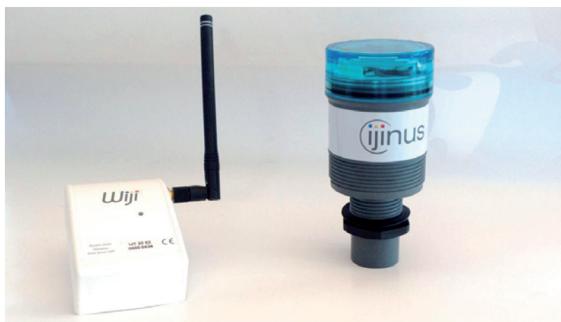
Figure 3: Ijinus ultrasonic sensor used as validation prototype.
